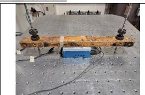
13. Mechanical Shock Test (-Z axis)
