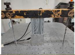
Mechanical Shock Test (-X axis)
