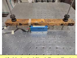
11. Mechanical Shock Test (-Y axis)
